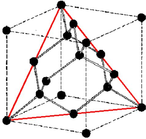
Silicon has a crystal lattice of the **diamond lattice** structure (see the schematic view on the left).
