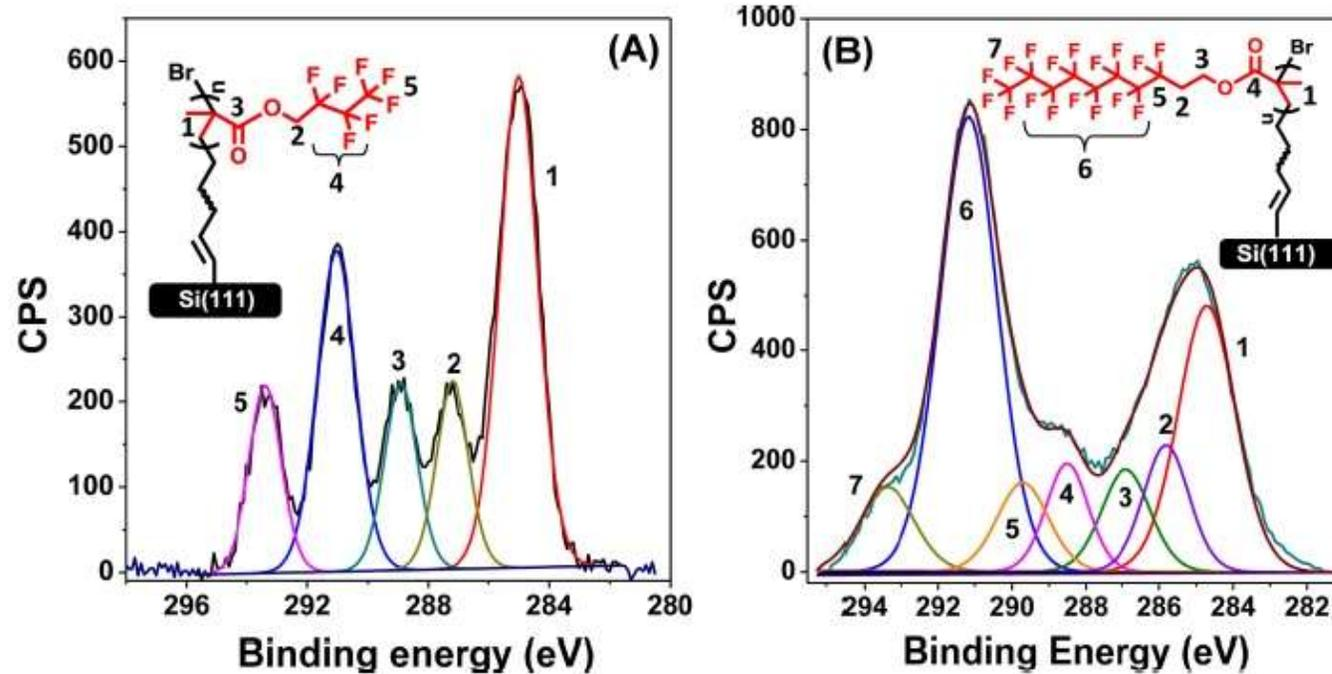
Figure 4. XPS C 1s spectra of SPF7 (A) and SPF17 (B) polymer brushes.
