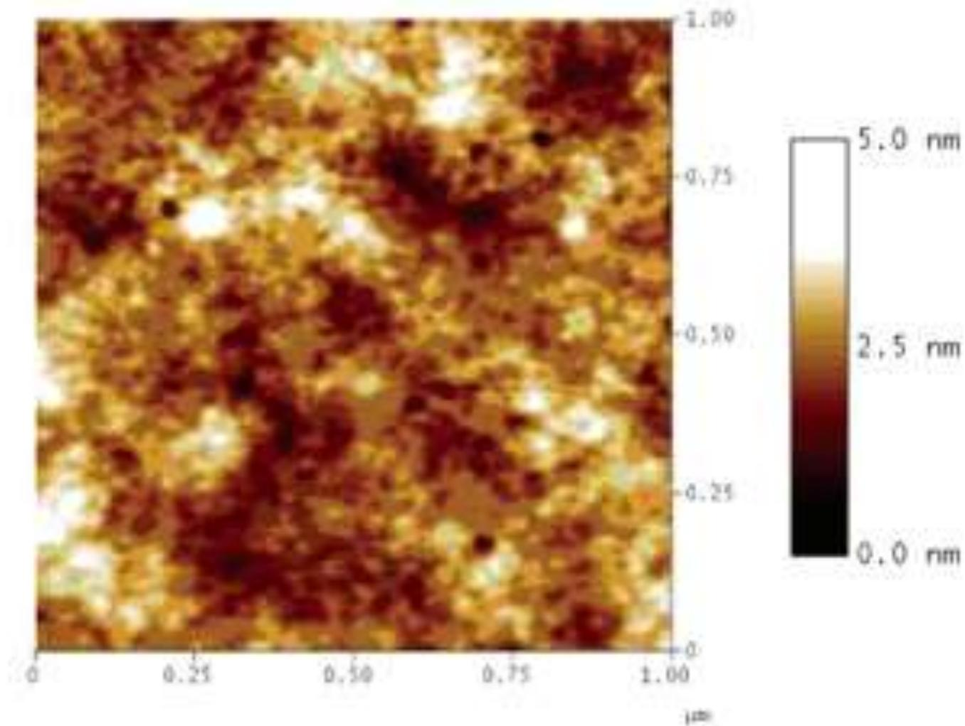
**Figure 2.** AFM 2D and 3D images ( $1 \mu\text{m}$  square) of poly(2-vinylpyridine) layer with 55 Å thickness, showing the topography of the surface used subsequently for SPR measurements. RMS roughness is 0.518 nm. The z-axis scale for the lower image is 5 nm per division.
