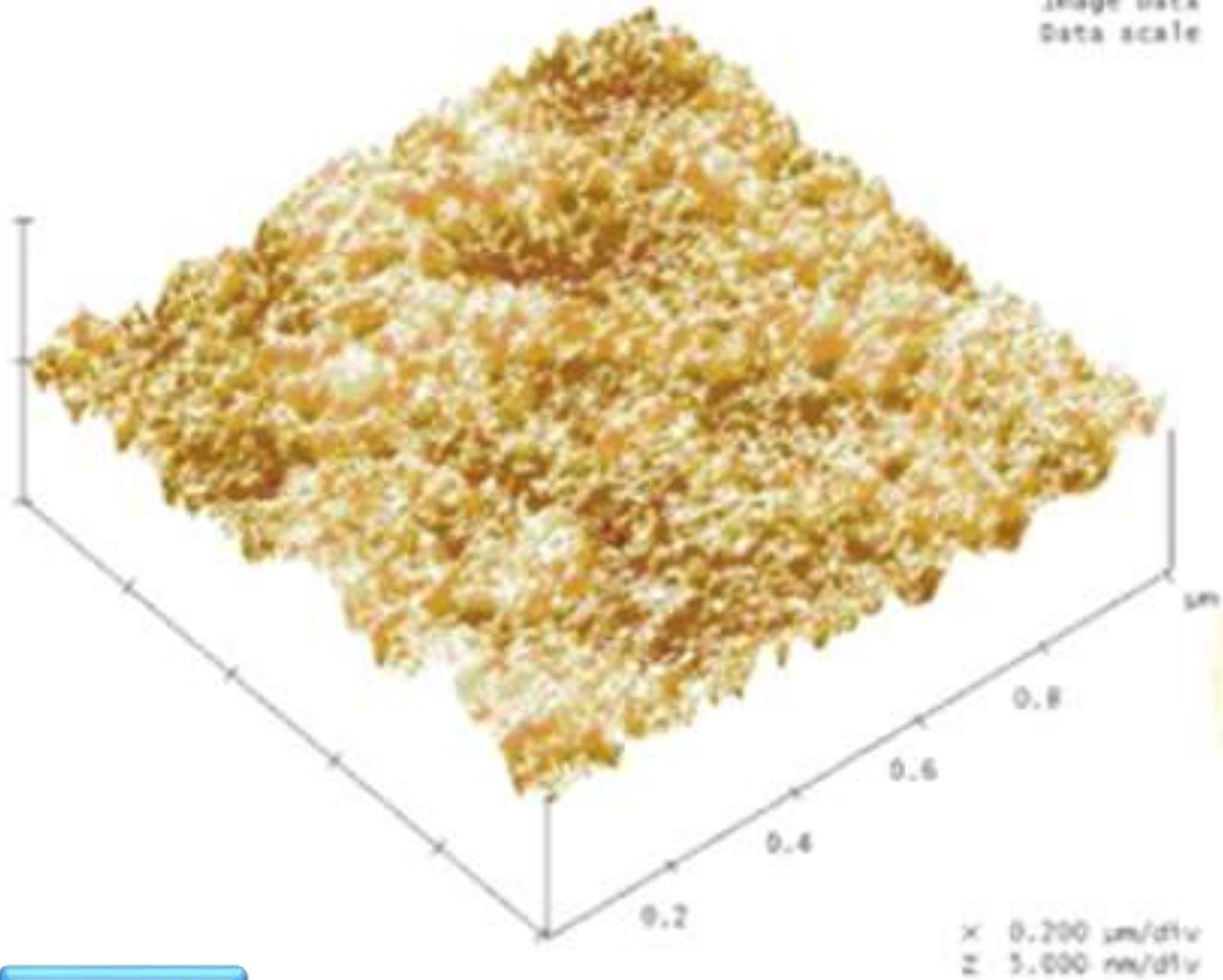
**Figure 2.** AFM 2D and 3D images ( $1 \mu\text{m}$  square) of poly(2-vinylpyridine) layer with 55 Å thickness, showing the topography of the surface used subsequently for SPR measurements. RMS roughness is 0.518 nm. The z-axis scale for the lower image is 5 nm per division.
