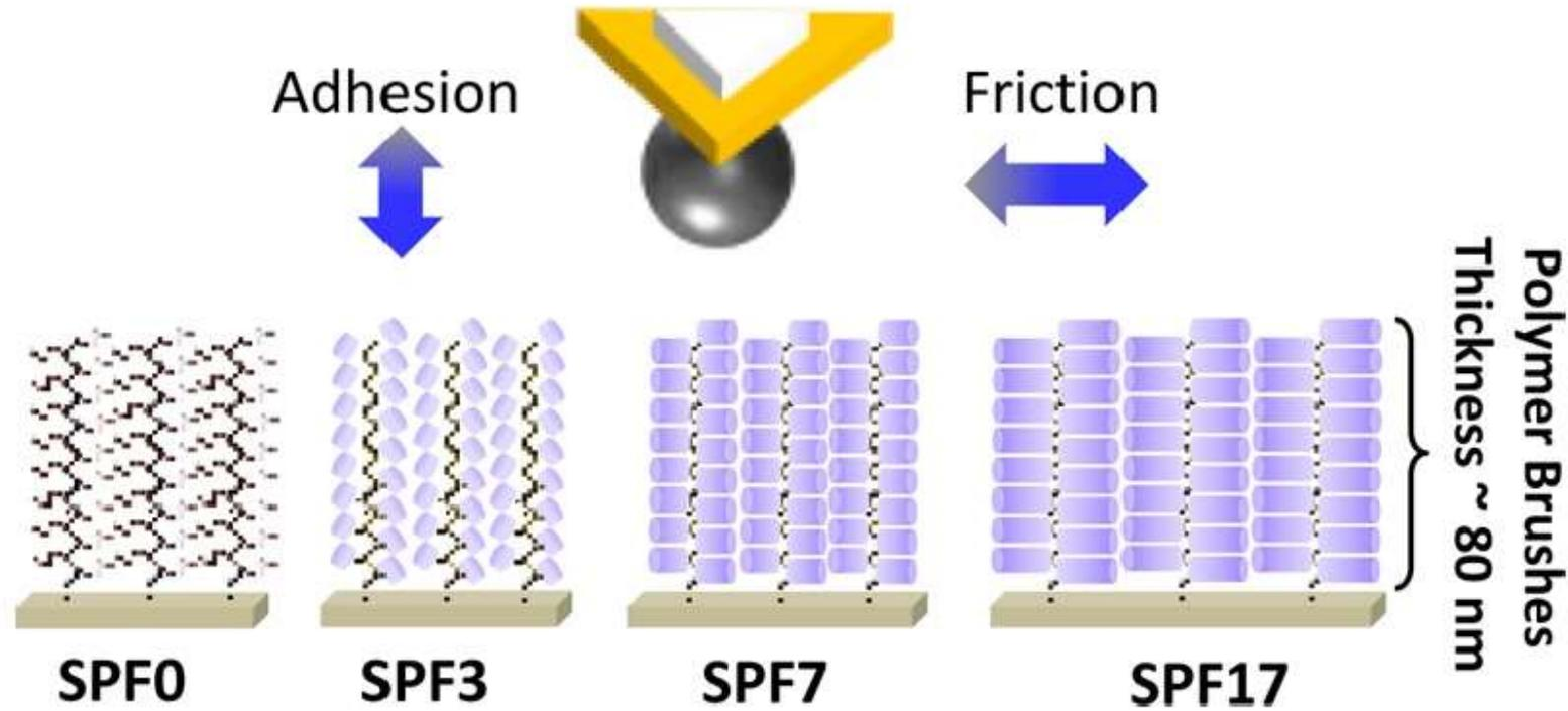
**Figure 1.** Schematic representation of covalently bound fluorinated polymer brushes at constant thickness ( $\sim 80$  nm) but with varying fluorine content to study the effects of fluorination in polymer on the adhesion and friction properties.
