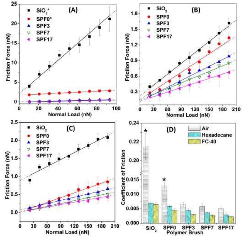
Figure 6. Friction forces versus applied normal load obtained under (A) ambient conditions (RH = 44 ± 2%) [\*dry conditions; RH < 5%], (B) in hexadecane, and (C) in FC-40. (D) Friction coefficient under all above conditions obtained from the slope of plots of the friction force versus normal load.
