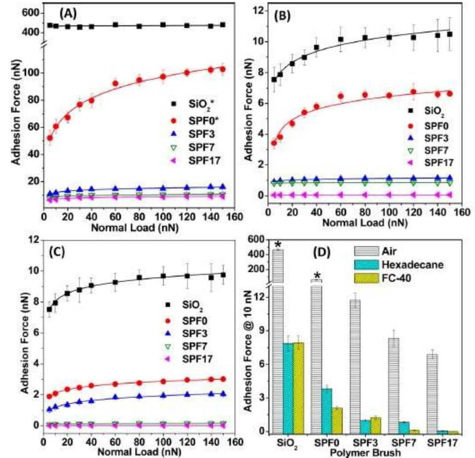
Figure 5. Adhesion (pull-off) forces at various applied normal load (5–150 nN) obtained on polymer brushes under (A) ambient (RH = 44 ± 2%) [\*dry (RH < 5%)], (B) hexadecane, and (C) FC-40. (D) Adhesion forces obtained at 10 nN applied normal load.
